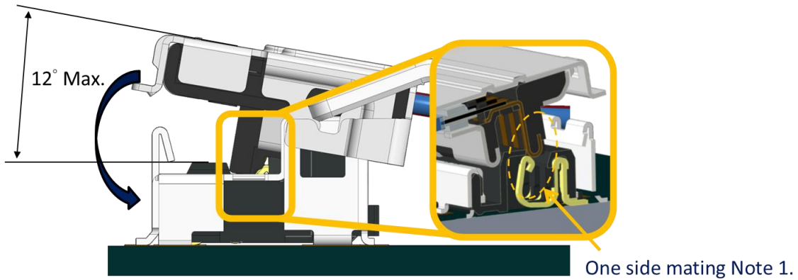
Fig.8 Insertion angle allowance
